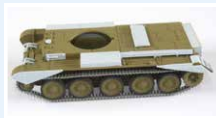
Photo 9 Track guards are also fitted to the front and rear.
