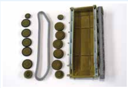
Photo 4 Twenty eight wheels and two tracks are all painted prior to assembly. The inner wheels are fixed to the axles, with the tracks being sandwiched between them and the outer wheels.
